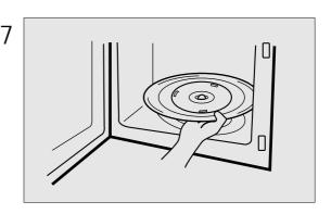
The roller guide and oven cavity floor should be cleaned regularly to avoid excessive noise. Simply wipe the bottom surface of the oven with mild detergent water or window cleaner and dry. The roller guide may be washed in mild sudsy water.
